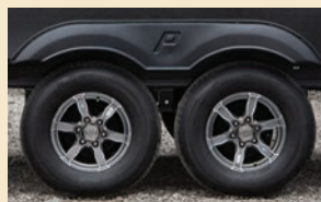
Aluminum wheels are optional. Standards include: Super Lube axles, ABS molded fender skirts and Lionshead nitro-filled tires for improved safety, tire life and fuel economy.
