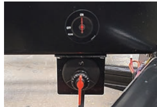
Seaflo battery isolator switch prevents power drain. Operates by removable key
